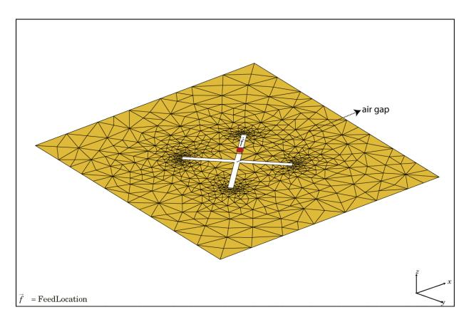
createFeed(antenna) plots a custom antenna mesh in a figure window. From the figure window, you can specify a feed location for the mesh and create a custom antenna. To specify a region for the feed point, select two points, inside triangles on either side of the air gap.
