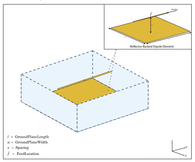
The infiniteArray class creates an infinite antenna array in the X-Y plane. Infinite array models a single antenna element called the *unit cell*. Ground plane of the antennas specifies the boundaries of the unit cell. Antennas without a ground plane require a reflector. By default, the infinite array has reflected-backed dipoles as antenna elements. The default dimensions are chosen for an operating frequency of 1 GHz.
