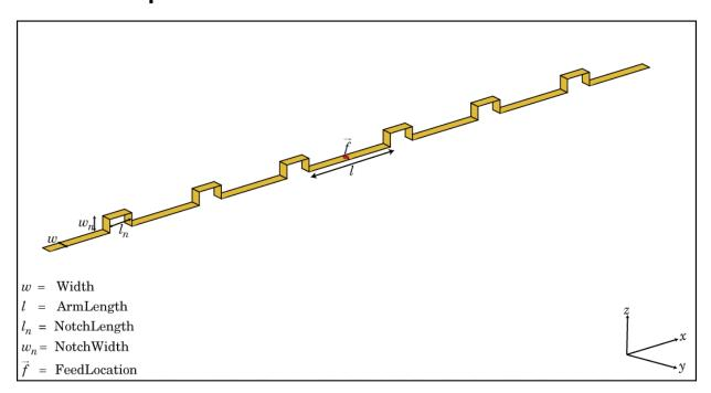
The dipoleMeander class creates a meander dipole antenna with four dipoles. The antenna is center fed and it is symmetric about its origin. The first resonance of meander dipole antenna is at 200 MHz.
