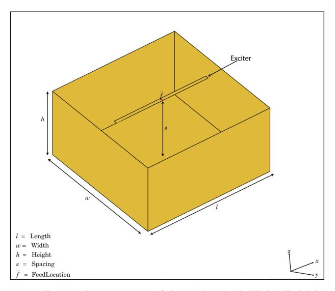
The cavity class creates a cavity-backed antenna located on the X-Y plane. The default cavity antenna has a dipole as an exciter. The feed point is at the origin.
