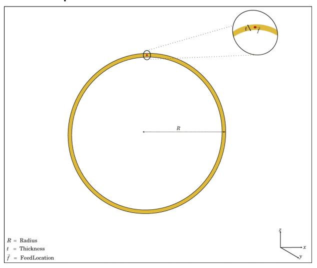
The loopCircular class creates a planar circular loop antenna on the X-Y plane. The thickness of the loop is related to the diameter of an equivalent cylinder loop by the equation
