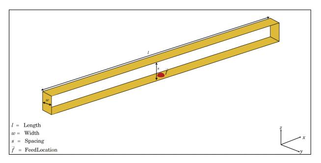
The dipolefolded class creates a folded dipole antenna on the X-Y plane. The width of the dipole is related to the diameter of an equivalent cylindrical dipole by the equation
