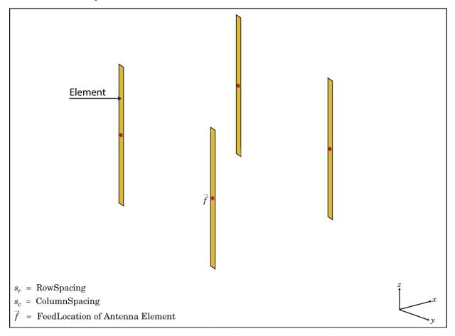
The rectangularArray class creates a rectangular antenna array in the X-Y plane. By default, the rectangular array is a four-element dipole array in a  $2 \times 2$  rectangular lattice. The dipoles are center-fed. Each dipole resonates at 70 MHz when isolated.
