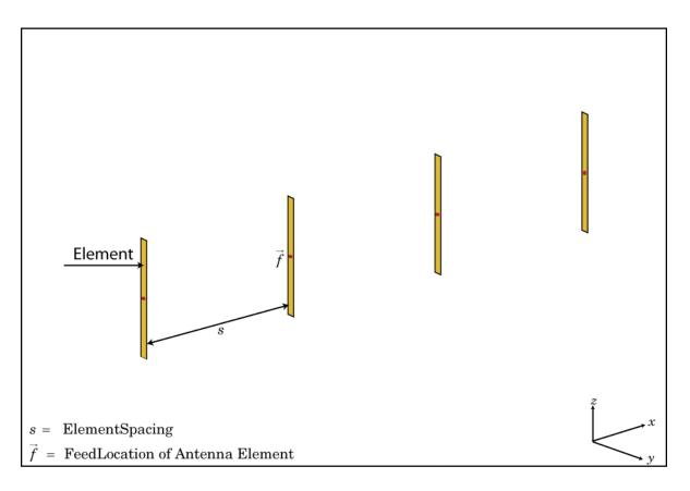
The linearArray class creates a linear antenna array in the X-Y plane. By default, the linear array is a two-element dipole array. The dipoles are center fed. Each dipole resonates at 70 MHz when isolated.
