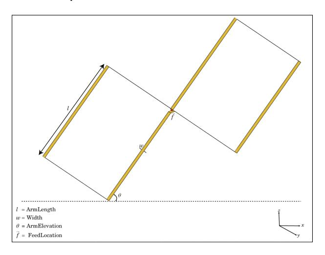
The biquad class creates a biquad antenna. The antenna is center fed and symmetric about its origin. The default length is chosen for an operating frequency of 2.8 GHz. The width of the strip is related to the diameter an equivalent cylinder:
