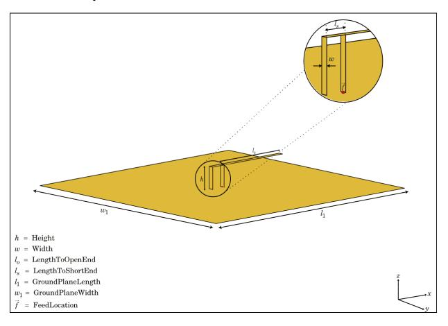
The invertedF class creates an inverted-F antenna mounted over a rectangular ground plane. The width of the metal strip is related to the diameter of an equivalent cylinder by the equation
