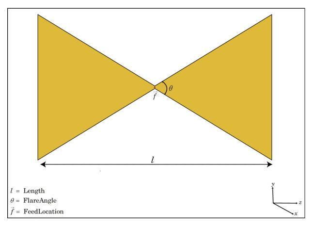
The bowtieTriangular class creates a planar bowtie antenna on the Y-Z plane. The default planar bowtie dipole is center-fed. The feed point coincides with the origin. The origin is located on the Y-Z plane.
