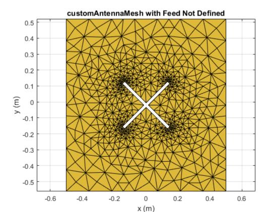
Create the feed for the custom antenna across the points (0.07,0.01) and (0.05,0.05) meters respectively.
