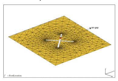
The customAntennaMesh class creates an antenna represented by a 2-D custom mesh on the X-Y plane. You can provide an arbitrary antenna mesh to the Antenna Toolbox and analyze this mesh as a custom antenna for port and field characteristics.
