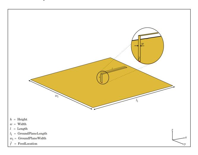
The invertedF class creates an inverted-L antenna mounted over a rectangular ground plane. The width of the metal strip is related to the diameter of an equivalent cylinder by the equation
