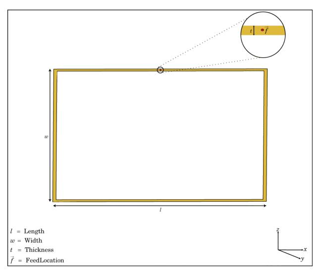
The loopRectangular class creates a rectangular loop antenna on the X-Y plane. The thickness of the loop is related to the diameter of an equivalent cylinder loop by the equation
