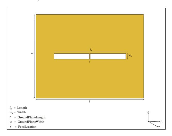
The slot class creates a rectangular slot antenna on a ground plane. The default slot has its first resonance at 130 MHz.
