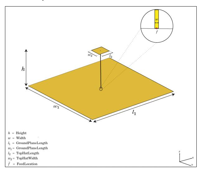
The monopoleTopHat class creates a top-hat monopole antenna mounted over a rectangular ground plane. The monopole always connects with the center of top hat. The top hat builds up additional capacitance to ground within the structure. This capacitance reduces the resonant frequency of the antenna without increasing the size of the element.
