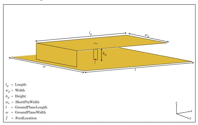
The pifa class creates a planar inverted-F antenna. The default PIFA antenna is centered at the origin. The feed point is along the length of the antenna.
