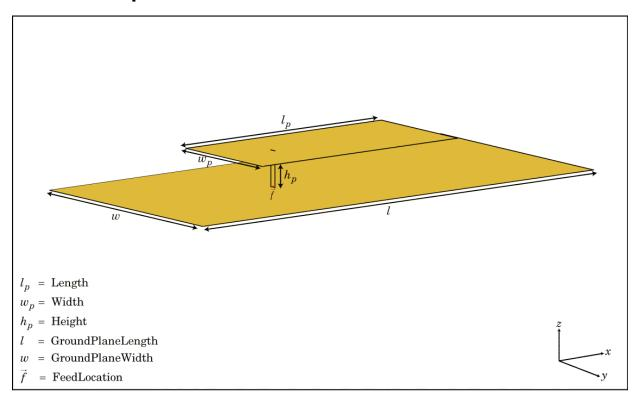
The patchMicrostrip class creates a microstrip patch antenna. The default patch is centered at the origin. The feed point is along the length of the antenna.
