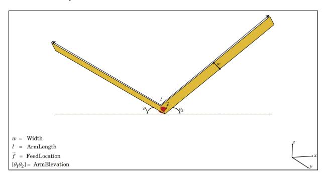
The dipoleVee class creates a planar V-dipole antenna in the X-Y plane. The width of the dipole is related to the circular cross-section by the equation
