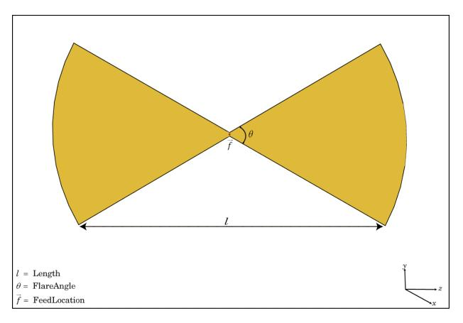
The bowtieRounded class creates a planar bowtie antenna, with rounded edges, on the Y–Z plane. The default rounded bowtie is center fed. The feed point coincides with the origin. The origin is located on the Y-Z plane.
