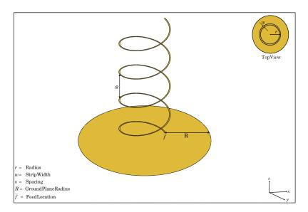
The helix class creates a helix antenna on a circular ground plane. The helix antenna is a common choice in satellite communication.
