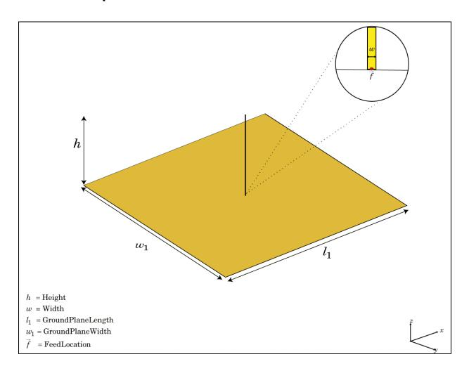
The monopole class creates a monopole antenna mounted over a rectangular ground plane. The width of the monopole is related to the diameter of an equivalent cylindrical monopole by the equation
