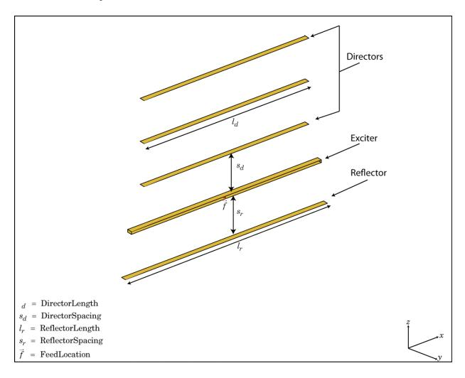
The yagiUda class creates a classic Yagi-Uda array comprised of an exciter, reflector, and *N*- directors along the z-axis. The reflector and directors create a traveling wave structure that results in a directional radiation pattern. The exciter, reflector, and directors have equal widths and are related to the diameter of an equivalent cylindrical structure by the equation
