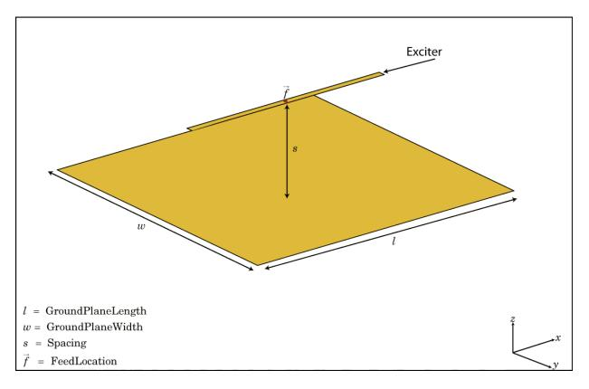
The reflector class creates a reflector-backed antenna located on the X-Y plane. The default reflector antenna uses a dipole as an exciter. The feed point is at the origin.
